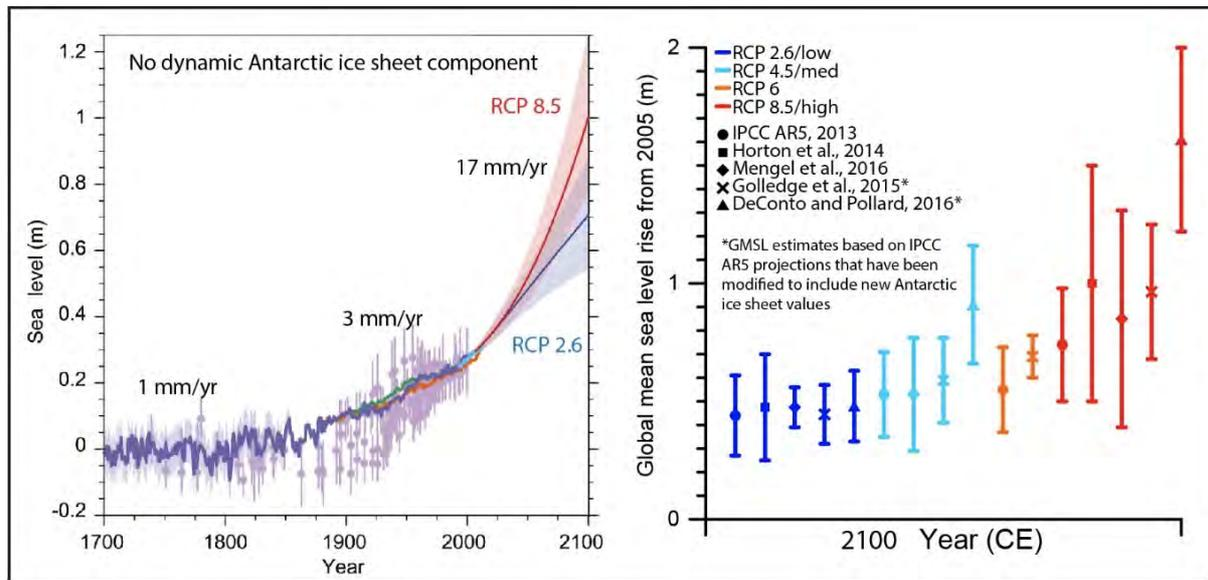
**Figure 2:** Left - Sea level projections to 2100 from IPCC AR5. Centre - Sea level projections at 2100 updated to include dynamic response of Antarctic Ice Sheet.
