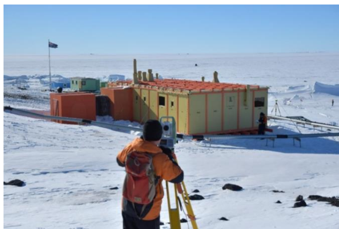
Deformation survey of TAE 1 Hut, Pram Point, on 7 November 2019 Photo: Christopher Stephens
