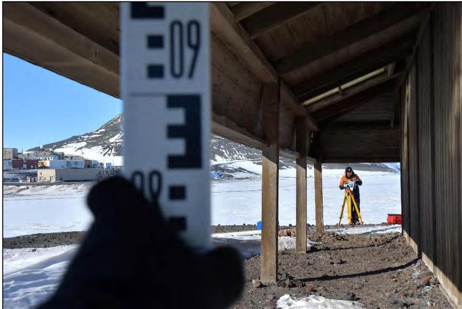
Deformation survey of Discovery Hut, Hut Point, on 7 November 2019
