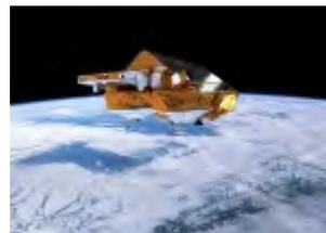
CryoSat's radar altimeter detects tiny variations in the height of the ice across the entire continent, including on the steeper continental margins where the vast majority of ice losses occur.
