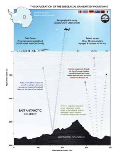
Fig. 2.8-2. Methods in the exploration of the subglacial Gamburtsev Mountains. (Image: British Antarctic
