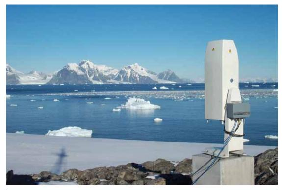
Fig. 3.5-4. Vaisala CT25K cloudbase recorder at Rothera (U.K.). (Photo: Jon Shanklin)
