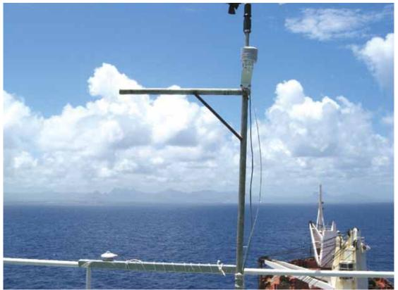
Fig. 5.3-6. Weather parameters were recorded along the ship track by using an Automatic Weather Station installed on onboard MV *Emerald Sea* during the 26th Indian Scientific Expedition to Antarctica (2006–2007) for IPY project no. 70. (Photo: Luis Alvarinho)
