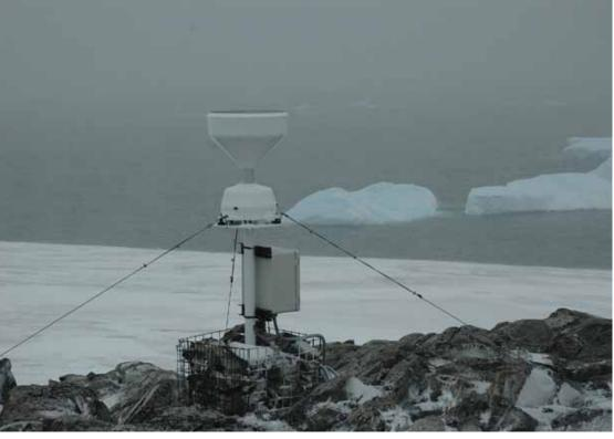
Fig. 3.5-5. A modern aerodynamic automatic tipping bucket gauge at Rothera (U.K.). It doesn't work well in Antarctica, particularly in light snow or strong wind, and needs a shield. (Photo: Jon Shanklin)
