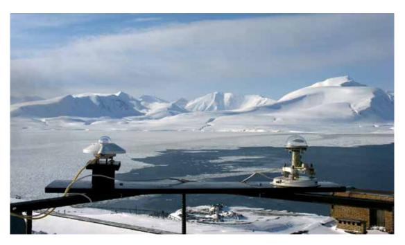
Fig. 2.1-2. Yanishevsky-Savinov (right) and Kipp and Zonen (left) pyranometers used in intercomparisons carried out at the Russian station Barentsburg (Svalbard) in April 2008. (Photo: Boris Ivanov; Ivanov et
