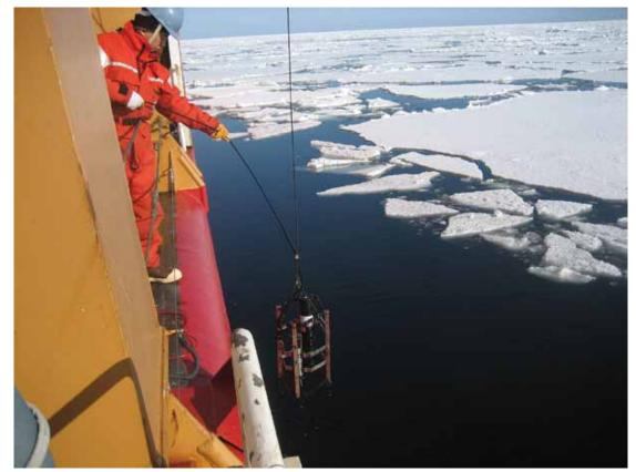
Fig.5.3-3. Water optics observation in northern Bering Sea conducted from the U.S. icebreaker *Healy*. (Photo: Jinping Zhao)
