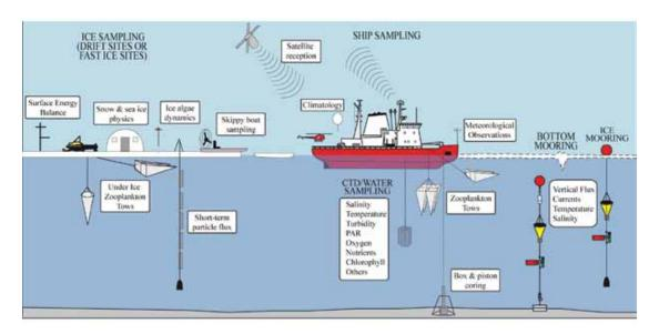
Fig. 2.2-17. Schematic of the scientific equipment used on the Amundsen and at ice camps nearby.
