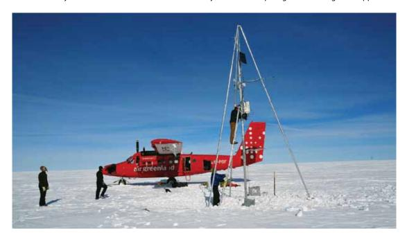
Fig. 2.4-2. Deploying an automatic weather station on the Greenland ice sheet during IPY. (Photo: K. Steffen)
