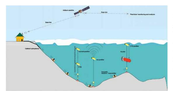
Fig. 3.2-8. A potential means of achieving a difficult but climatically-important measurement at modest cost. Through cooperation with the Canadian Defense Research Development Corporation (DRDC), it is planned to use an acoustic/cable/ satellite link to provide oceanographic data from Barrow Strait in (Image: Simon Princenberg BIO)
