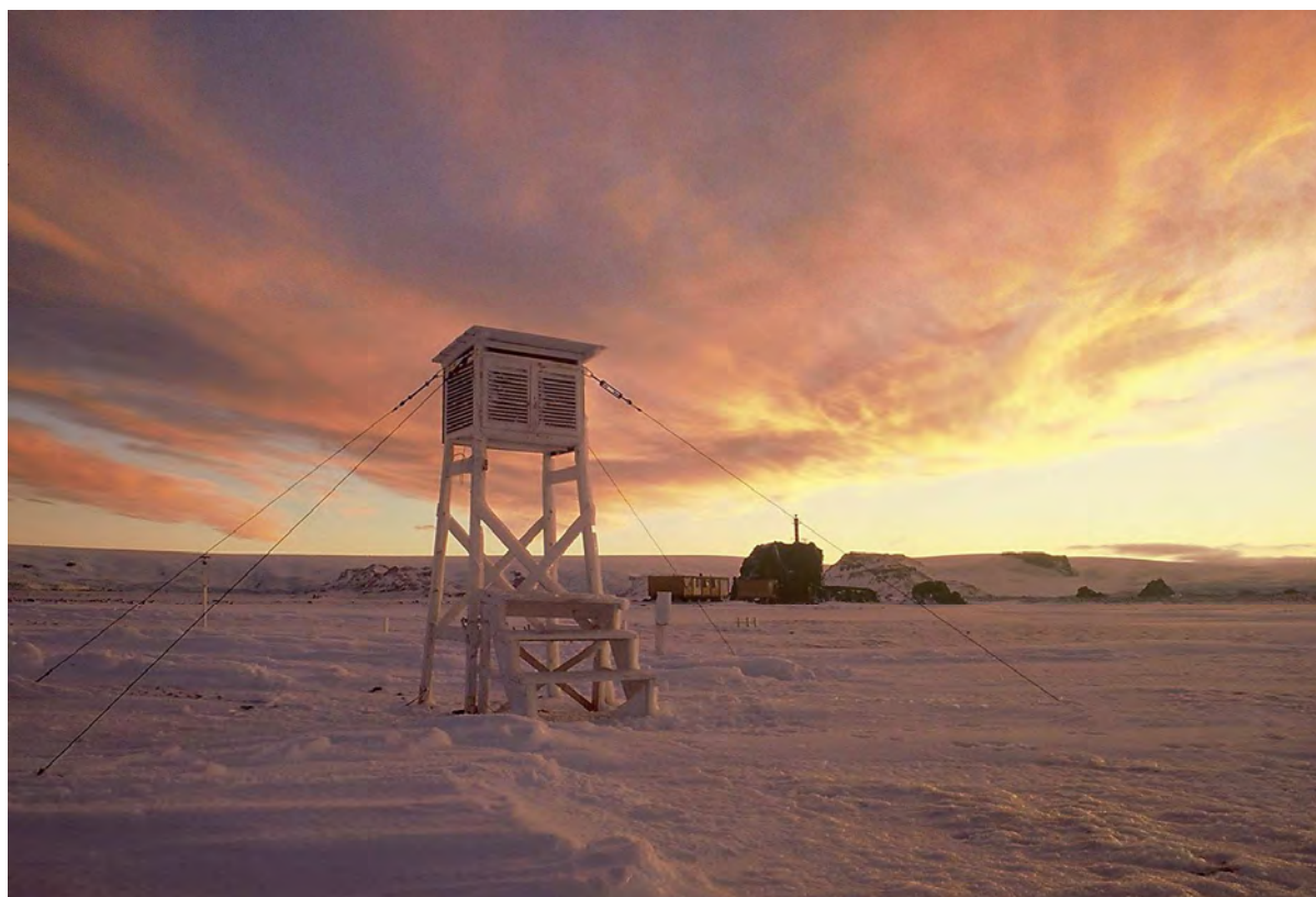
Standard meteorological screen in winter conditions at the Polish Arctowski Station, King George Island.
