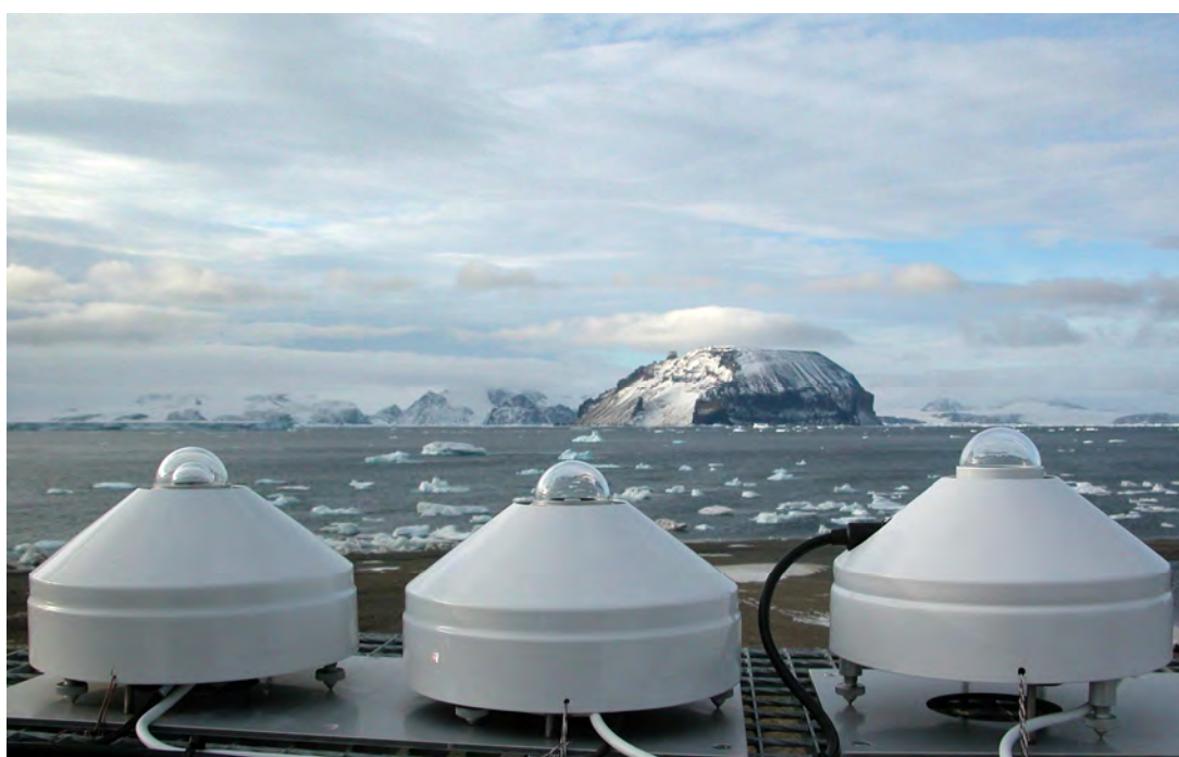
Broadband radiometers installed at the Czech J. G. Mendel Station (James Ross Island).
