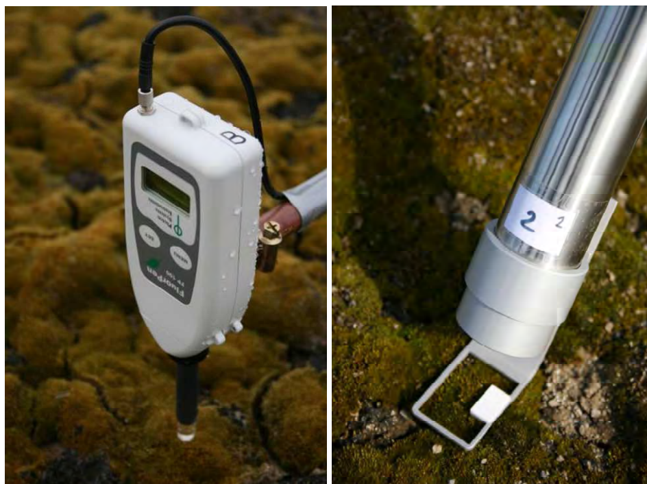
Two types of fluorometers installed temporarily (left) or permanently (right) over a moss cushion ( Bryum sp.) at experimental field plot located close to a seashore of James Ross Island.
