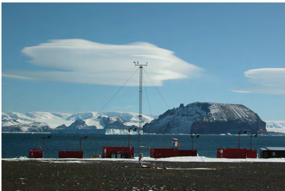
Meteorological tower with the array of wind sensors at the Czech J. G. Mendel Station (James Ross Island).
