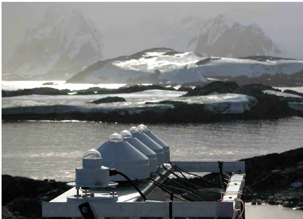
Radiometers equipped with the ventilation units installed on a special platform at the Ukrainian Vernadsky Station (Galindéz Island, western Antarctic Peninsula).
