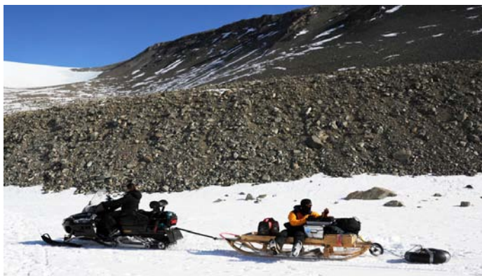
Figure 2. Acquisition of ice thickness profiles of a frozen lake in the Sør Rondane Mountains, using an ice radar.
