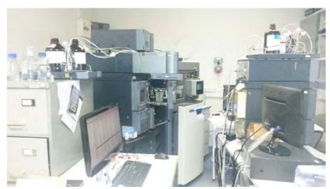
Figure 1. Complete set-up of UPLC-MS using an auxiliary pump system for improved compound detection; Stellenbosch University, Central Analytical Facilities, MS-Lab.
